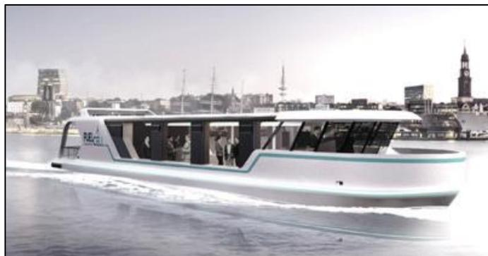
applies to this HyMeth-Ship is simple but involves an extremely complex construction. Methanol is reformed to hydrogen, which is then burned. The CO<sub>2</sub> thus created will be stored and later reconverted into methanol.
