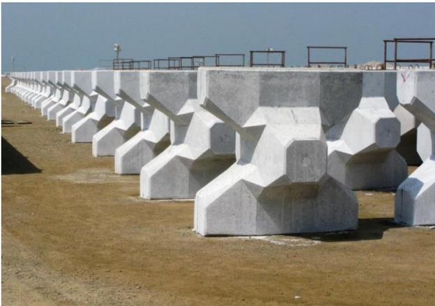
Figure 7 - Accropode™ units stored ready for transport to the breakwaters.
