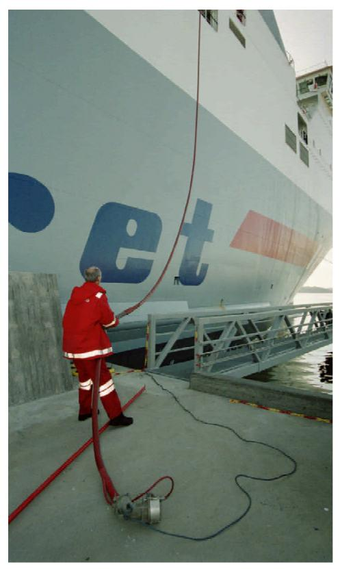
It is easy to connect the vessel. It only takes a couple of minutes to make the electrical connection and switch off the ship's engine, here one of Cobelfret's vessels.
