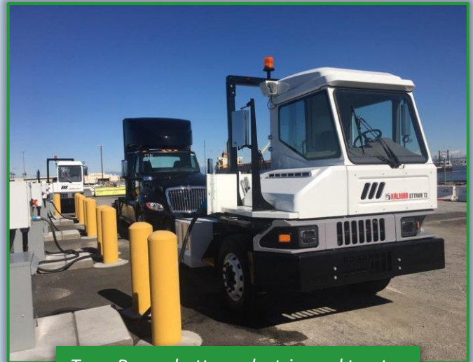
TransPower battery-electric yard tractor
