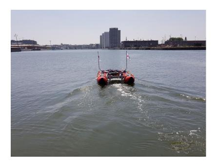
One of the Port Authority's responsibilities is inspection and maintenance of the maritime infrastructure, including the beds of the docks. Regular measurements of the water depths at the berths and at all other points are carried out, both to ensure safe passage and mooring for ships and
