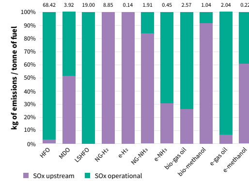
Figure 13 - Net oxides of sulphur emissions
