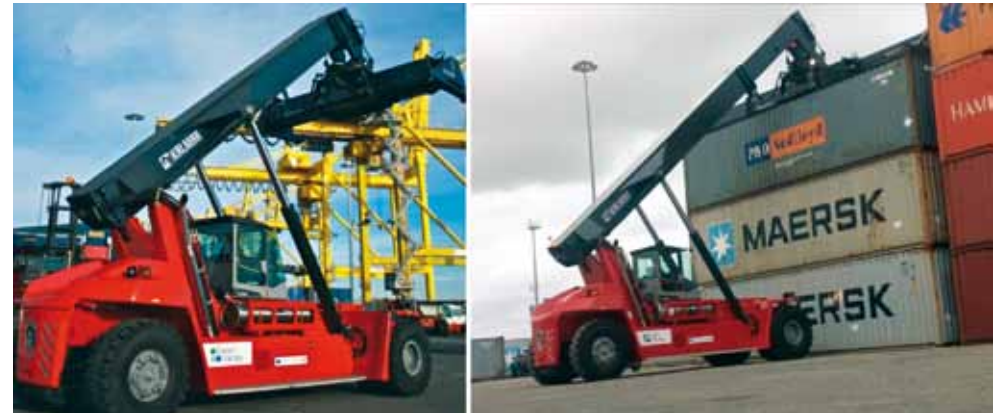
Figure 49. LNG Reach Stacker Prototype Working at Amerigo Vespucci Interporto and Livorno Darsena Toscana
