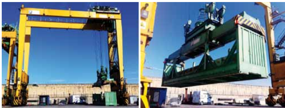
Figure 42. RTG Operating with 15L Displacement Gen-Set
