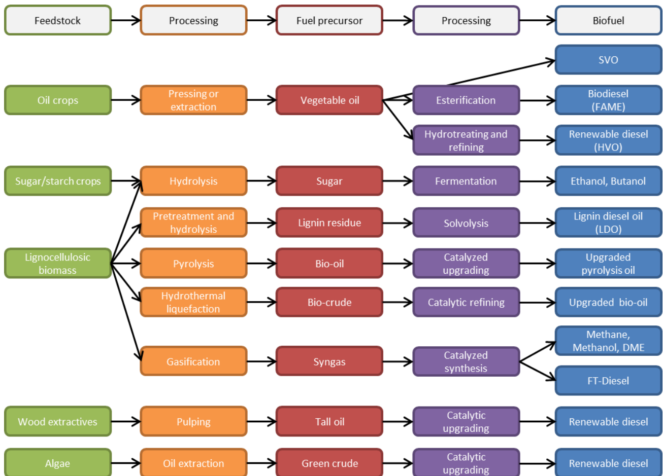
Figure 2: Biofuel production technologies
