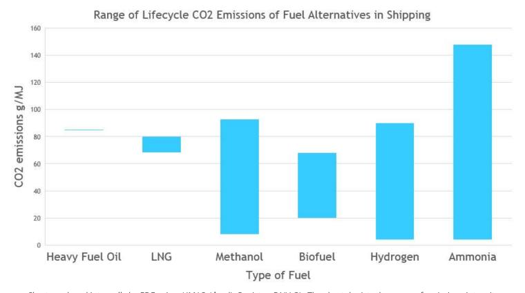
Chart produced internally by EDF using: UMAS, Lloyd's Register, DNV GL. The chart depicts the range of emissions intensity from the different potential fuel types for shipping
