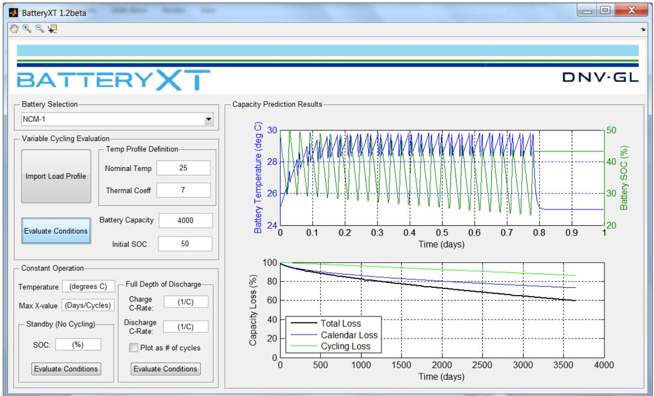
**Figure D.2. Screenshot of Battery XT, showing user inputs which allow them to evaluate any chosen battery chemistry for any given application profile.**
