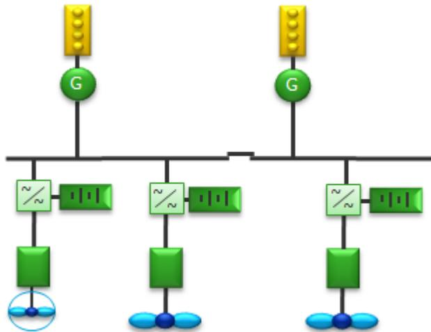
**Figure 3.10 Hybrid battery propulsion with distributed batteries**
