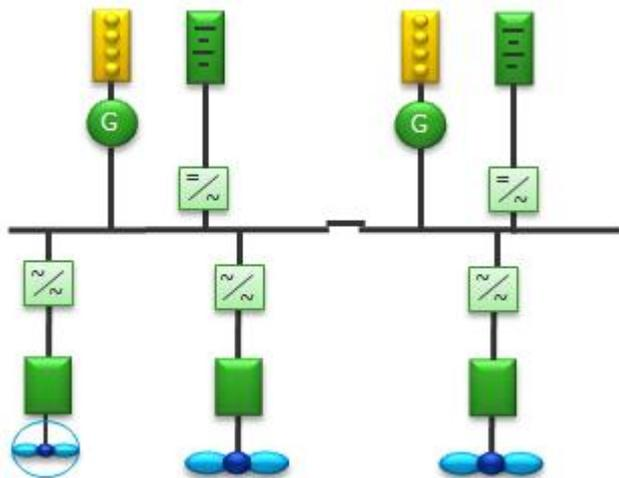
**Figure 3.9 Battery hybrid propulsion**
