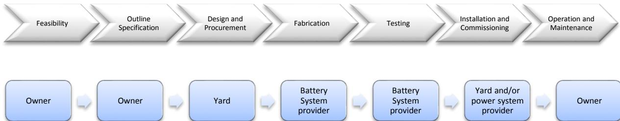
**Figure 4.1. The battery system in the shipbuilding process and the responsible party**
