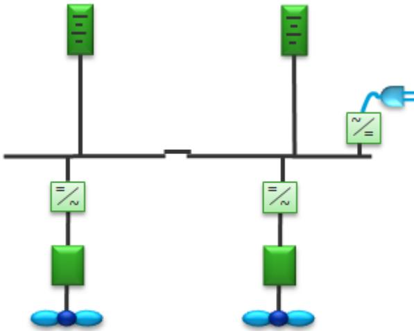
**Figure 3.12 Battery propulsion for an all electric ship**
