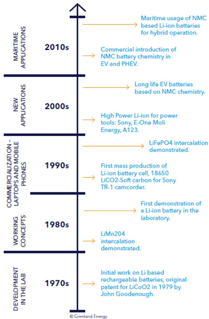
**Figure 3.1 Milestones of lithium-ion battery technology**
