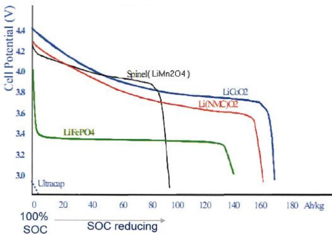
**Figure 3.4 Cell voltage as a function of SOC is an important feature for controls and power production**
