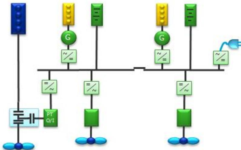
**Figure 3.11 Power system with electrical/mechanical hybrid solution, battery hybrid with plug in possibilities and a DC distribution**
