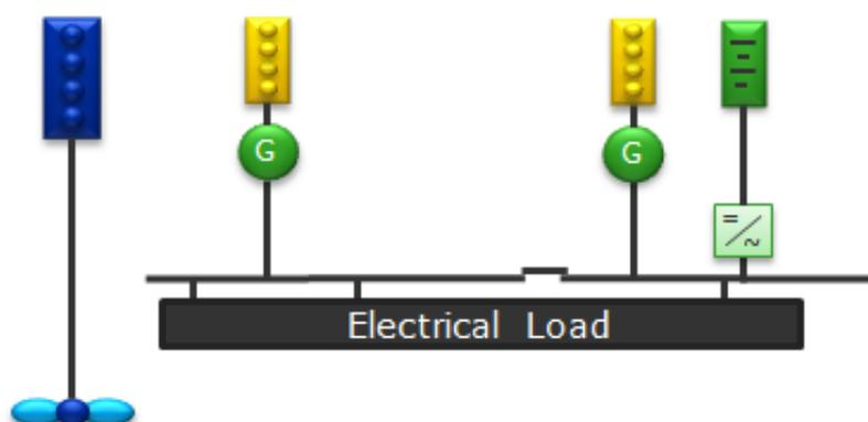
**Figure 3.8 Mechanical propulsion with battery hybrid electric power plant**
