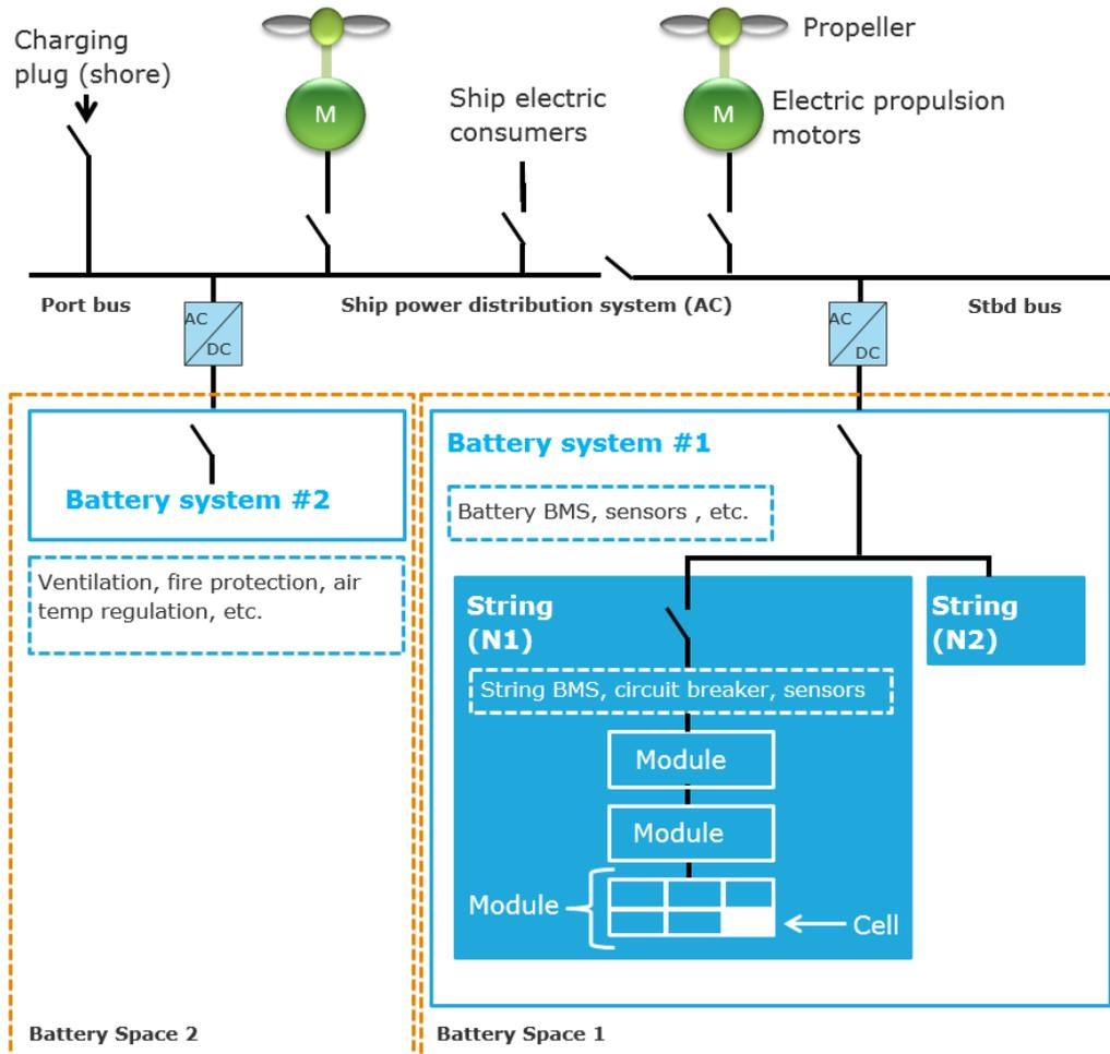
**Figure B.1. Battery System and related sub-systems**
