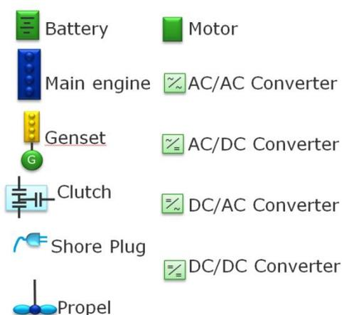
**Figure 3.7 Symbols for electric components. In this report, "Genset" means the engine and generator set. For the converters, a transformer may be added to minimize noise that can influence the BMS or battery system.**
