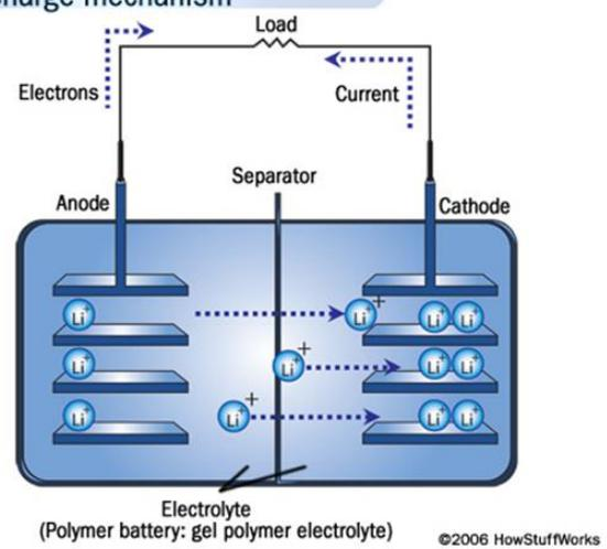
**Figure 3.3 Basic principles and components of a lithium-ion battery**
