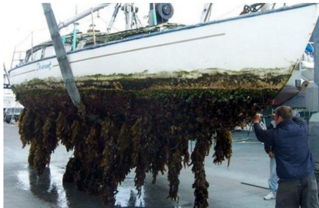
630 Figure 10: Fouling costs upon the attachment to ship hull which cause serious problems in shipping industry. Reproduced with permission from Editec Group.
