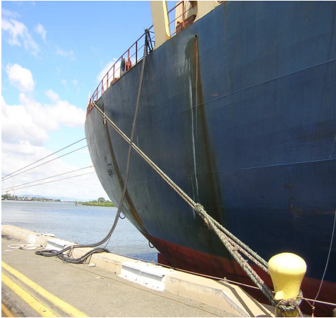
Figure III-7: Shore-side power connection at the USS POSCO facility in Pittsburg, CA.
