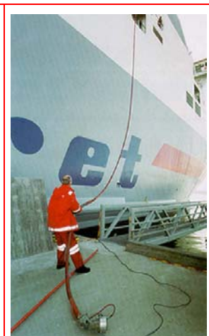
Figure B7 A single main cable for the power supply and manoeuvre is all that is needed to connect the ship.
