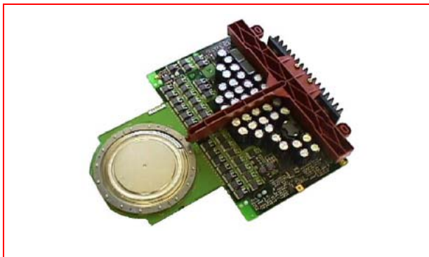
Figure D9 Single IGCT block unit.
