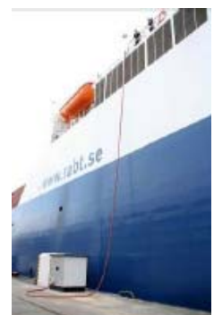
Figure B14 One cable, supplied by the ship, is connected to the cabinet.
