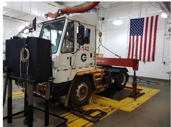
Hybrid truck on the dynamometer
