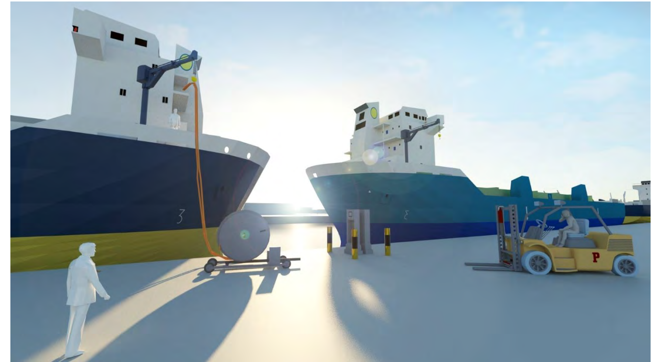
Figure 4—11 3D render shore power connection process stage 2 - Cable reel lifting towards the ship side connection using the vessels onboard crane or quayside crane
