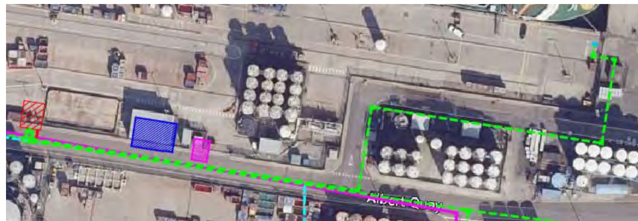
Figure 4—13 Proposed LV cabling route avoiding excavation of the reinforced concrete deck slab at Albert Quay.
