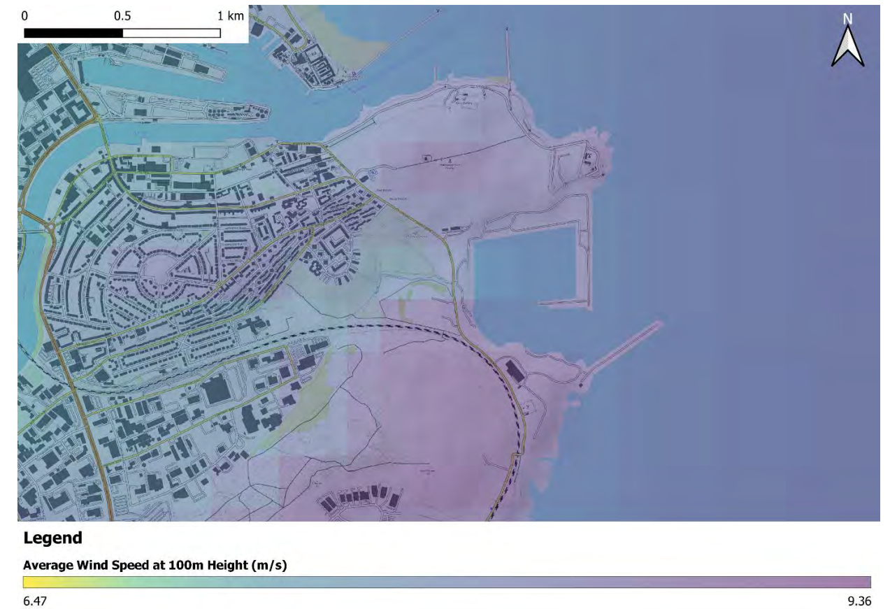
Figure 9—18 PoA south harbour wind speeds at 100m
