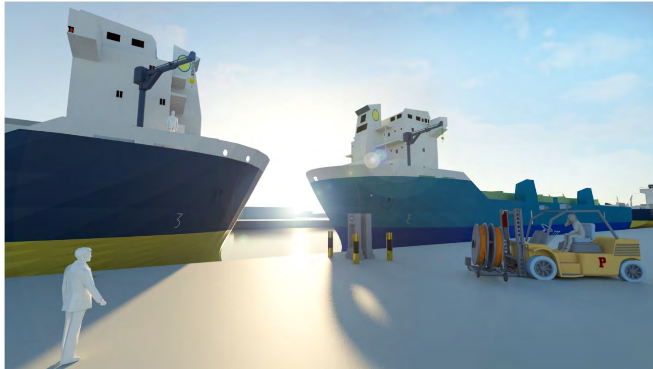
Figure 4—10 3D render shore power connection process stage 1 - Cable reel delivered to berthing area during the ship berthing process
