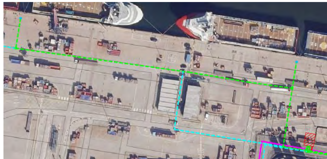
Figure 4—14 Proposed route in cyan may allow easier excavation. Based on available as-built drawings, there is a possibility that the surfacing in this area may be less substantial than the 275mm thick reinforced concrete slab present in the surrounding area.
