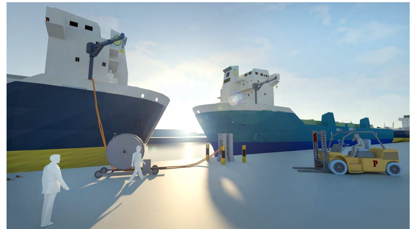
Figure 4—12 3D render shore power connection process stage 3 - Shore connection made with ship and fixed connection point
