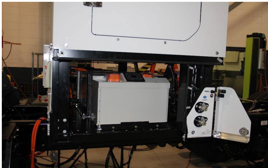
Figure 8. High-Voltage Battery Integrated into Hydrogen Storage Cabinet
