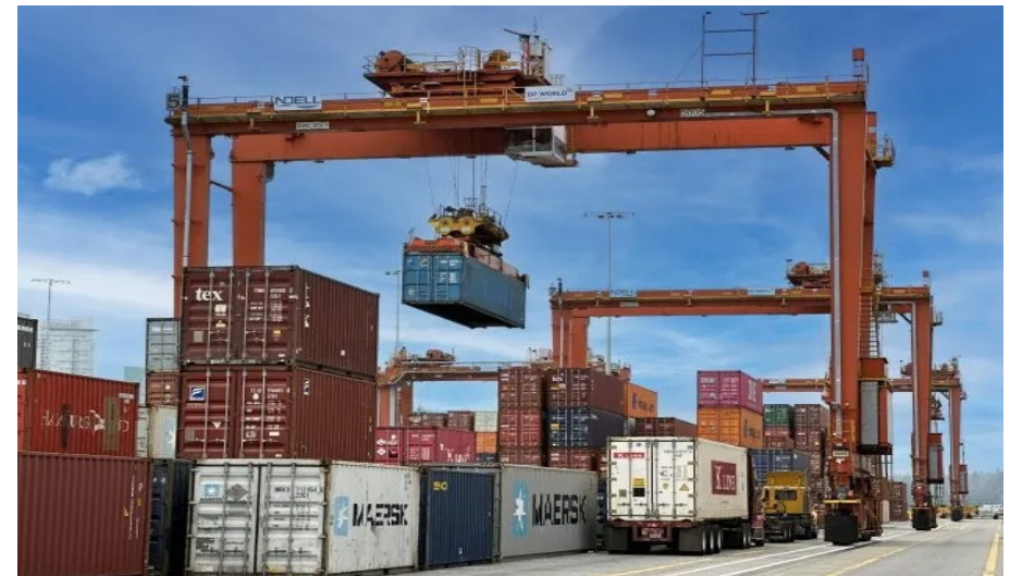
DP World Rubber-Tired Gantry Crane at The Port of Vancouver (CNW Group/TYCROP Manufacturing Ltd)
