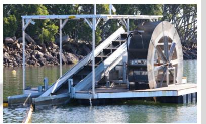
The project developed Solar Powered **Automatic River Cleaner** (SPARC) - a 24/7collection device that can be used in rivers to collect debris, lift it out of the water and place it in a bin, ready for removal.
