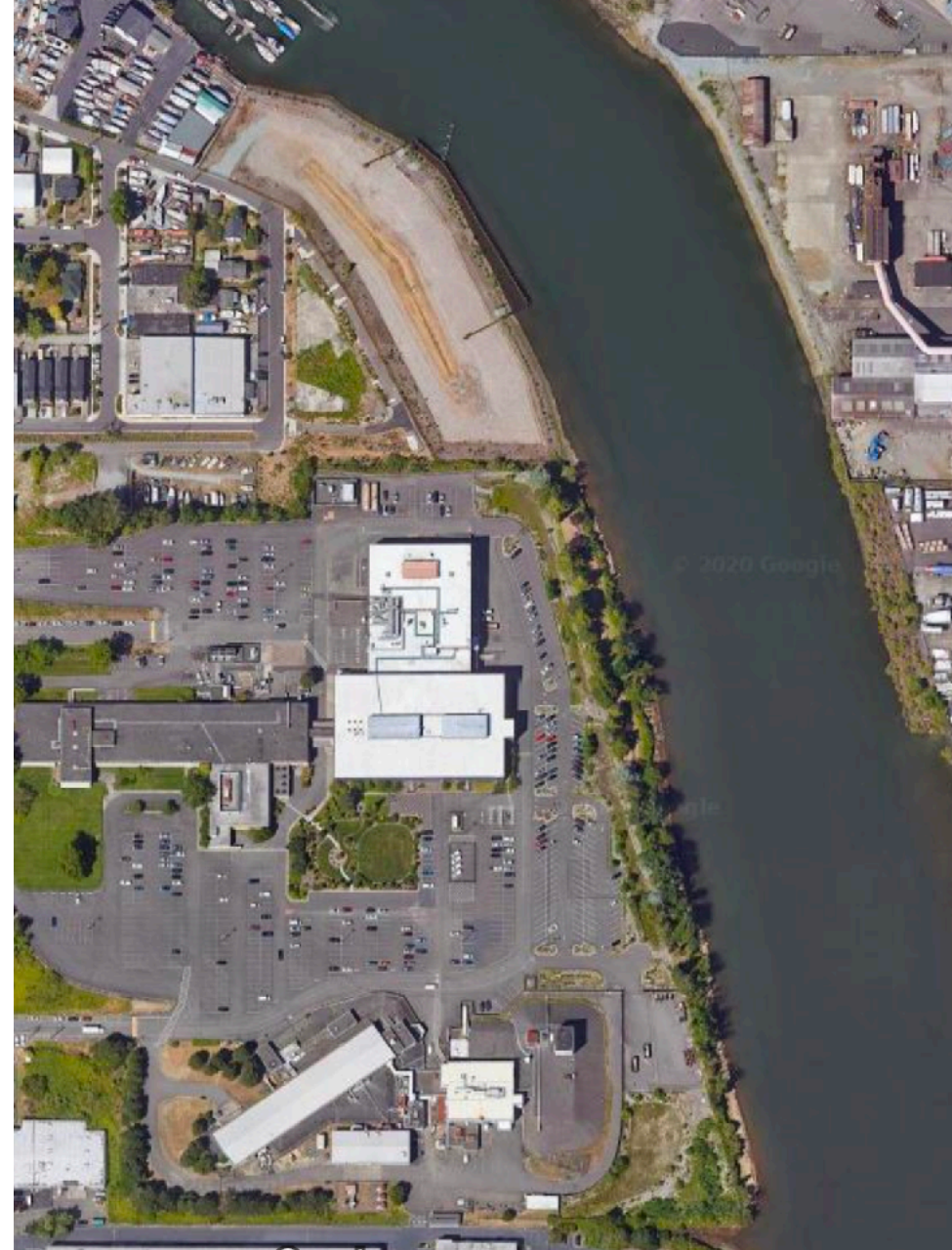
Google Map view of Terminal 117 project site and adjacent street right-of-way area following cleanup, 2019. Adjacent street improvements include pathways, seating, public art, interpretive information, native landscape vegetation, and green storm-water-infrastructure. The site is stable and ready for implementation of habitat and public access improvements.
