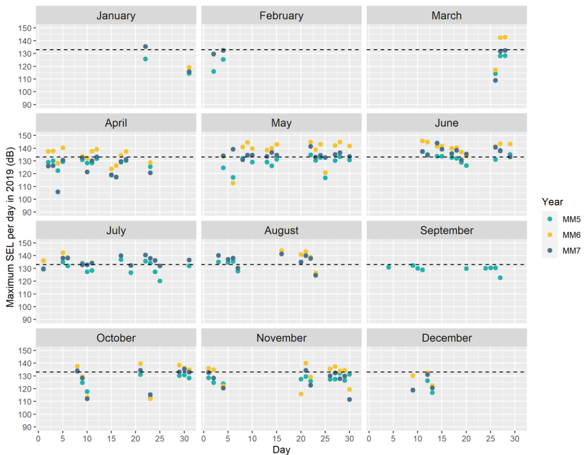
Figure 31. Maximum single-strike sound exposure level (SEL) per day, month and site (MM5, MM6 and MM7) in 2019, all of which are in the inner and mid harbour. The dashed line shows the behavioural threshold ( SEL = 133 \text{ dB re } 1 \mu\text{Pa}^2\cdot\text{s} ).
