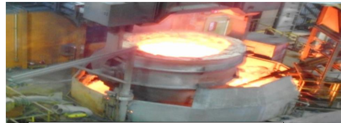
Desulfurizer in use
