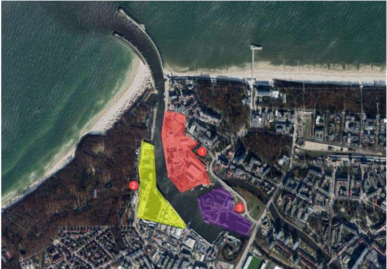
Figure 3-2. - Port of Kołobrzeg. Layout. (1) – cargo handling and administration area, (2) – fishing port and shipyard area, (3) – yacht marina
