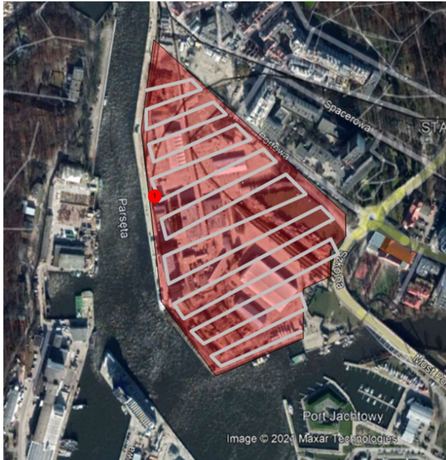
Figure 3-8. Preliminary mission plan for air quality monitoring
