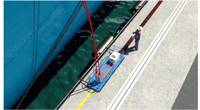
Connection point installed on top of autonomous vehicles w/ & w/o cable reel
