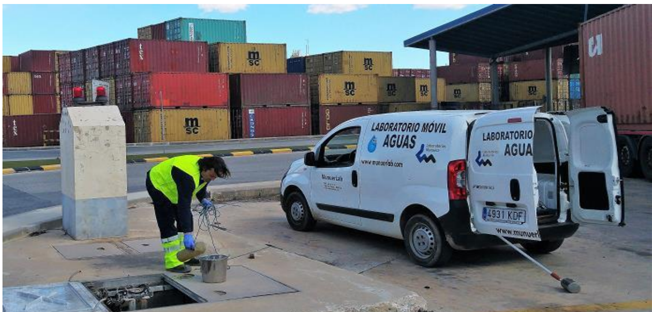
Sample collection from the pumping well at the Container Terminal in Santa Lucía
