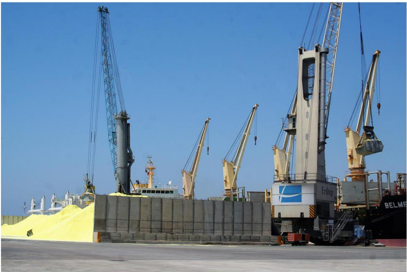
Solid bulk terminal at Escombreras' enlargement – Sulphur loading from Repsol Petróleo refinery
