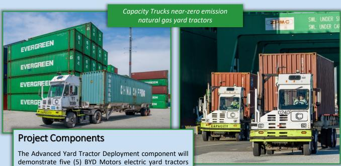
demonstrate five (5) BYD Motors electric yard tractors and twenty (20) Capacity Trucks near-zero emission natural gas yard tractors, fueled with renewable natural gas provided by Clean Energy Fuels.
