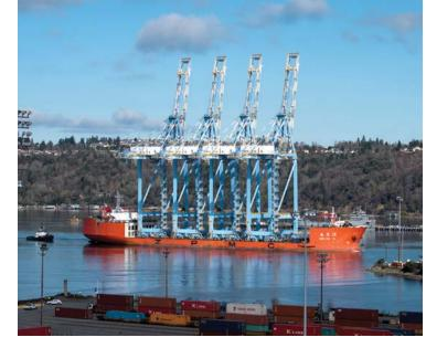
With an outreach of 24 containers, the new cranes are identical to the ones delivered in 2018 and are capable of serving ultra-large container vessels entering the trans-Pacific trade.
