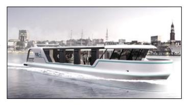
applies to this HyMeth-Ship is simple but involves an extremely complex construction. Methanol is reformed to hydrogen, which is then burned. The CO2 thus created will be stored and later reconverted into methanol.
